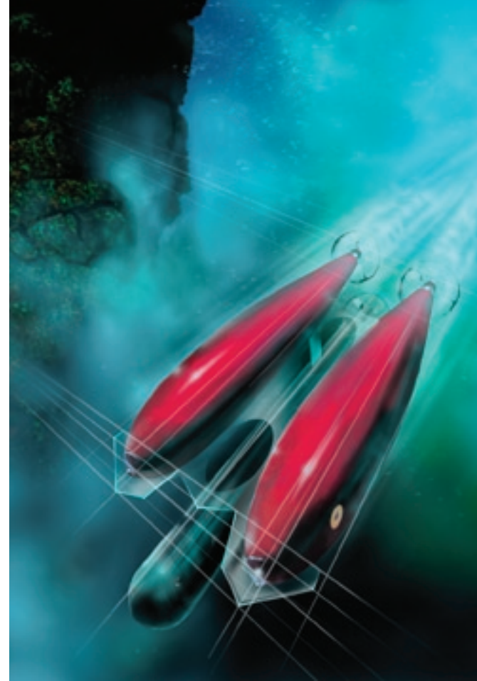
The Autonomous Benthic Explorer can navigate over the rugged terrain of the deep ocean, exploring the cooling lava of newly formed seafloor.
